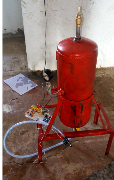
Fig.3diagram of Fuel injection testing equipment
