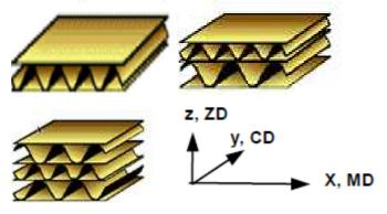
Fig. 1: Types of corrugated board a) Single wall b) Double wall Triple wall.
