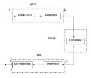
Fig.2 (a) Traditional Compression-then-Encryption (CTE) system.
