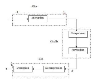
Fig.2 (b) Encryption-then-Compression (ETC) system.
