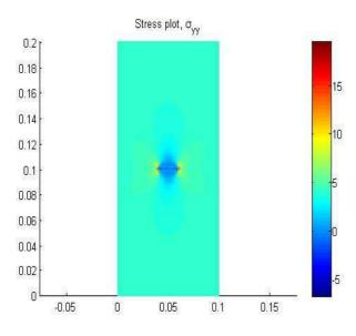
Fig. 3(a) Stress plot of  $\sigma_{yy}$  (MPa) during Combined loading
