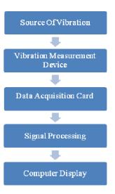
Figure: 1 Component of Architecture[8]
