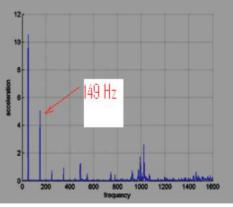
Figure 4 Outer race fault[1]
