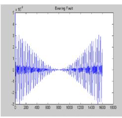
Figure 6 Time domain signal for faulty bearing[1]
