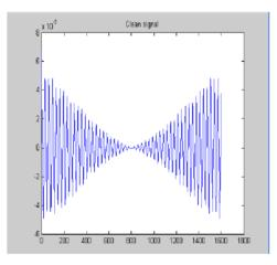
Figure 5 Time domain signal for healthy bearing[1]
