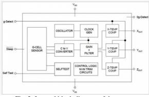
Fig. 2: Internal block diagram of the sensor.
