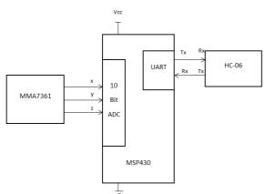
Fig. 1: Connection Diagram of the system
