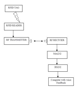
Fig.1: Block diagram of RFID technology
