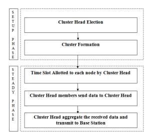
Figure 2: Workflow of the Proposed Protocol
