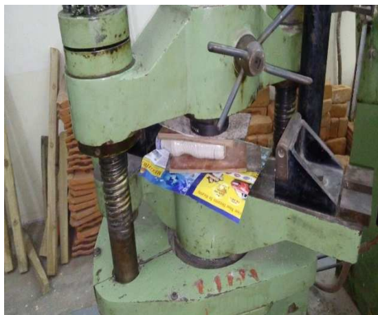
Fig. 3: Compression Test on Bottle filled with fly ash
