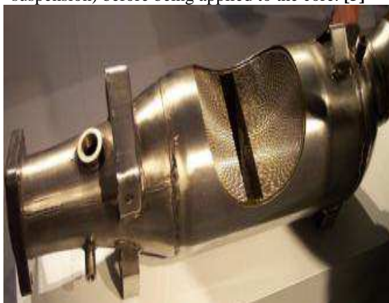
FIG.1: (a) Cutaway of a metal-core converter
