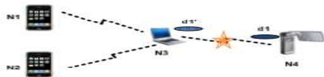
Fig1. Network partition due to link failure.
