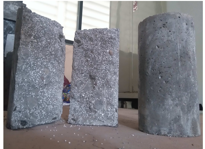
Fig 4- Cylinder after Split Tensile Test, Showing EPS beads Distribution.
