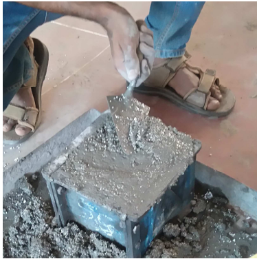
Fig 2 - Finishing the top surface of concrete mould.
