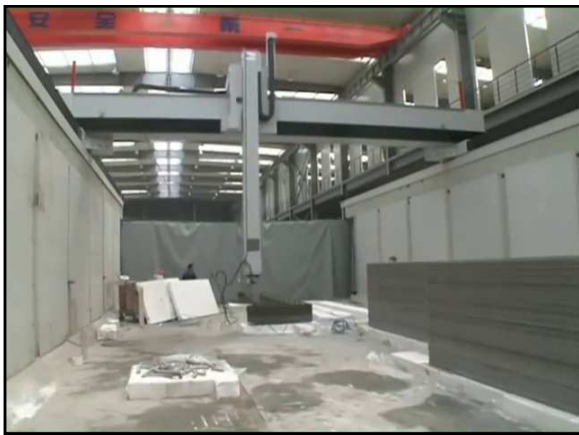
Fig. 7 The 3D printing Equipment used by WinSun Corporation, China
