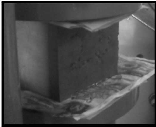
Fig.3. Hair Fibre Reinforced concrete cube with fewer cracks after compression test
