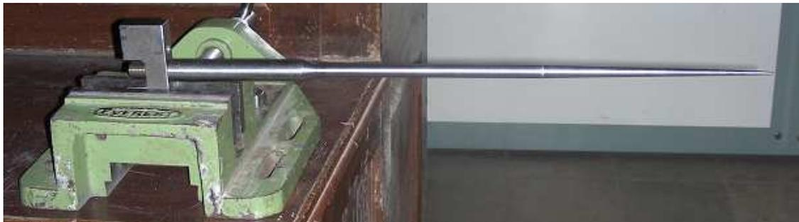
Fig. 4: Test Specimen (Scaled up dental pin) with fixture
