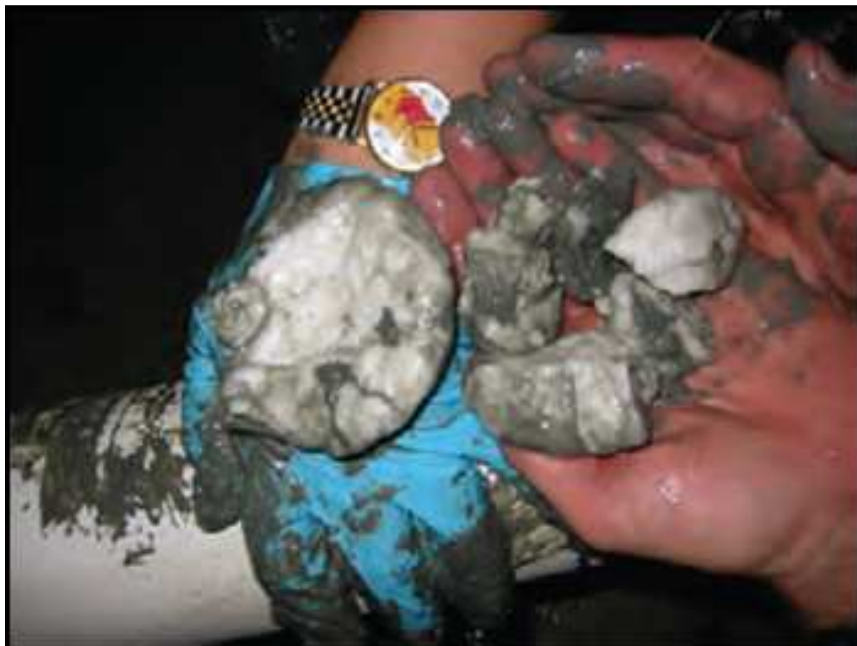
Figure 2: Sample of methane hydrate from the Gulf of Mexico. Methane hydrates can look like ice or packed snow but break down at atmospheric conditions, releasing nearly 160 times their own volume of methane gas. (Source : Photograph by W.J. Winters, U.S. Geological Survey)
