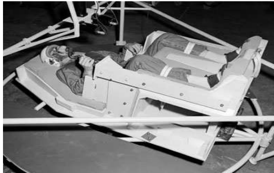
Fig.2: An astronaut sits in a spacecraft simulator in the zero-gravity position. Courtesy NASA
