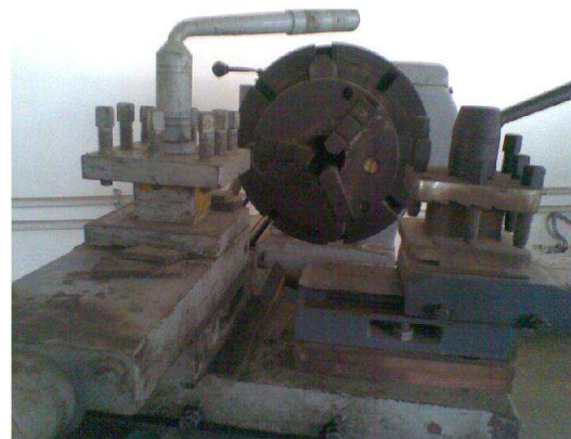
Fig. 7 Multi Tool Turning Setup
