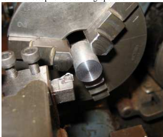
Fig. 6 Conventional Turning Setup
