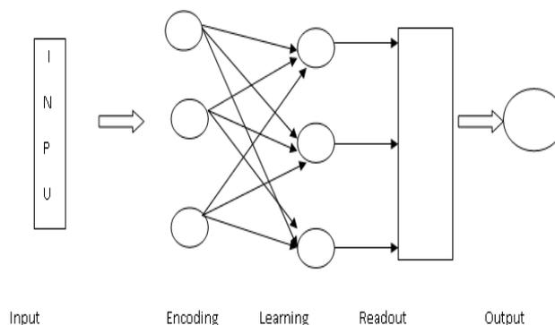
Fig 2: Architecture of Spiking Neural Networks
