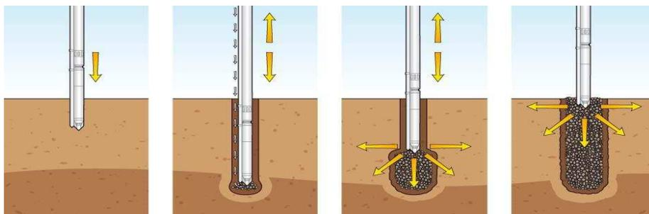
**Figure 2:** Dry – Bottom - feed method process schematic (Taube, 2001).
