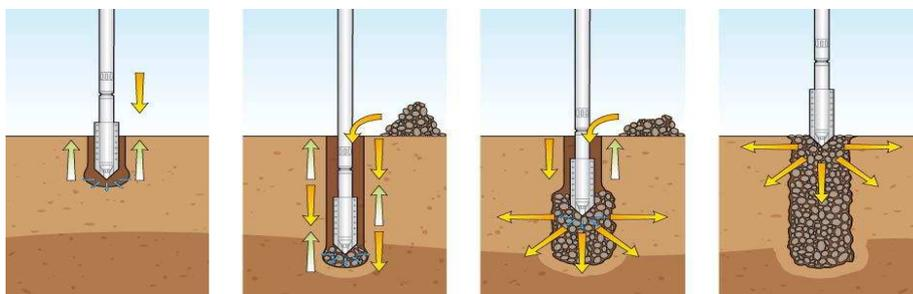
**Figure 3:** Wet - top - feed method process schematic (Taube, 2001)
