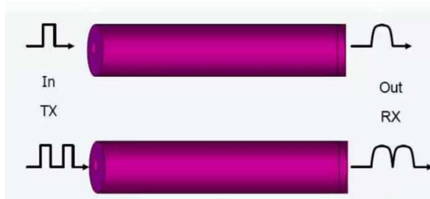
Fig.1. Chromatic dispersion causes pulse broadening and bit error
