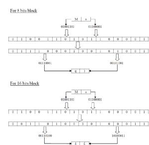
Figure 3: The encryption steps for the given example
