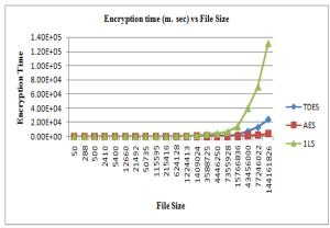
Figure 4:Graphical Representation of encryption times against file size in logarithmic scale
