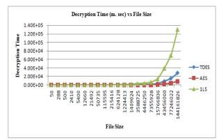
Figure 5:Graphical Representation of decryption times against file size in logarithmic scale
