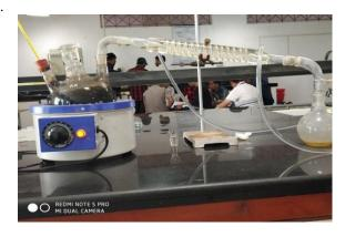
Fig 2: Vacuum Distillation Unit
