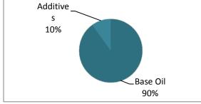
Fig 1.1: Composition of lubricant oil.
