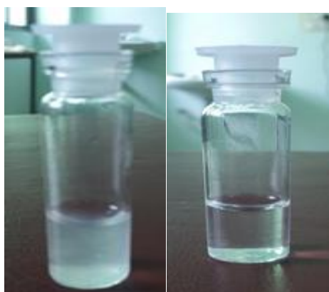
Fig 5: (a) Guar gum with solvent (b) after addition of cross linker STMP
