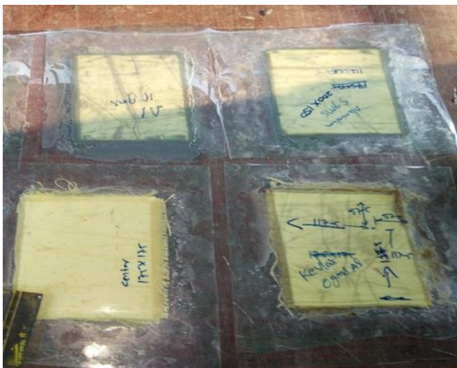
Fig 1: Fabricated hybrid composite materials with varying different proportions of filler material (Al).
