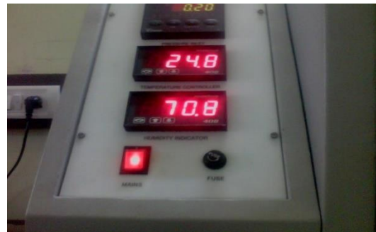
Fig.3. Readings of R/H Generator and Calibrator
