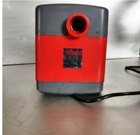
Fig. 7: Centrifugal Water Pump
