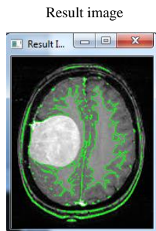
Fig. 7. Processed images after implementing Canny algorithm.
