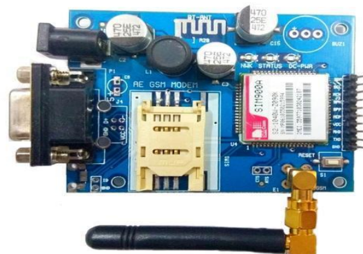
Figure 3: GSM/GPRS SIM900A Module
