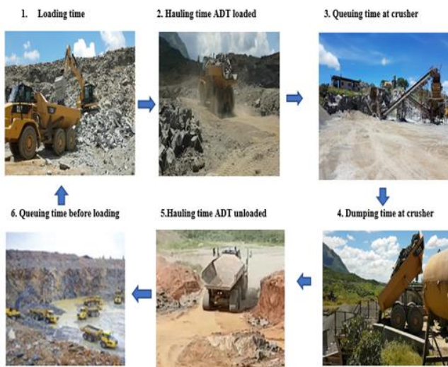
Fig. 3: Illustration of shovel-truck cycle time at Njuli quarry
